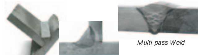
High-Deposition Fillet Welds
