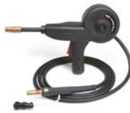
Magnum 100SG Spool Gun Designed to easily feed 4 in. (102 mm) diameter 1 lb. (0.45 kg) spools of .030 in. (0.8 mm) or .035 in. (0.9 mm) diameter SuperGlaze® aluminum MIG wire. Includes gun, adapter kit, .035 in. (0.9 mm) contact tips (qty. 3), gas nozzle, and a 1 lb. (0.45 kg) spool of SuperGlaze® 4043 .035 in. (0.9 mm) MIG wire. Packaged in a convenient carrying case. Order K3269-1
