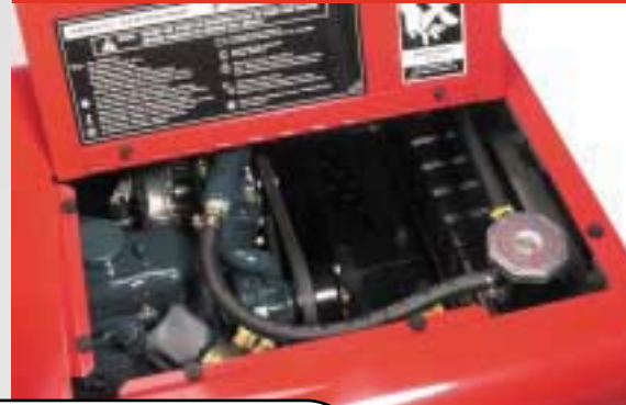
Easy Access Maintenance Panel to Engine & Water
