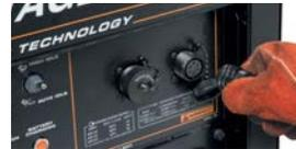
Output automatically switches to remote mode when remote device is connected. For the CC-stick, downhill pipe and Touch Start TIG® modes, the machine output dial becomes a maximum current limit for more fine tuning with the remote control dial or Amptrol™.
