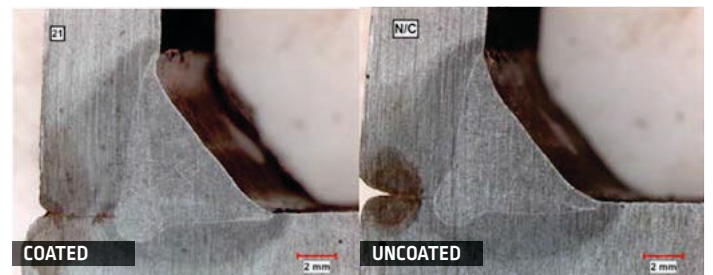
Micro-Etch testing shows no discernible weldment differences between uncoated & RP6 coated base material
