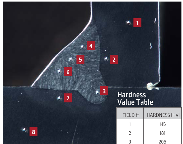
Cross sectional analysis displays a defect free fillet weld with robust hardness values
