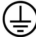
The frame of the welder must be grounded. A ground terminal marked with the symbol is located at the bottom of the input box for this purpose. See your local and national electrical codes for proper grounding methods.
