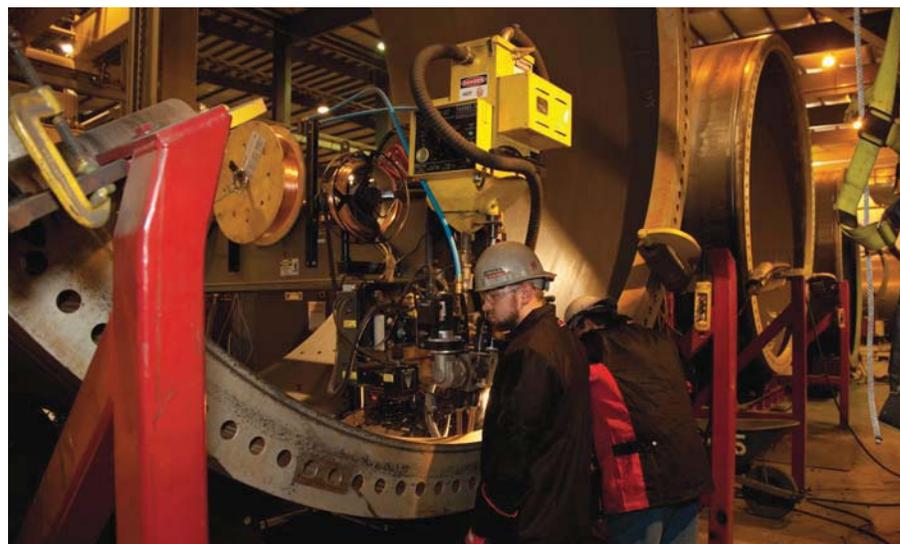
**FIGURE 2** Because wind towers are fabricated in segments, a lot of welding is needed to join them together. It is estimated that welders at Katana Summit, Columbus, Neb., used roughly 9,000 lbs. of welding wire and flux to join the four sections comprising the Cleveland wind tower.
