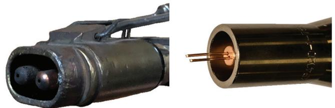
Figure 1. Tandem (left) and twin wire GMAW (right) processes
