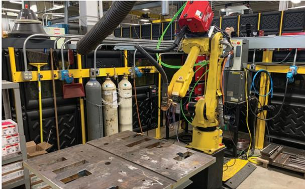
Figure 2. Lincoln HyperFill™ robotic TW-GMAW system installed in EWI's lab.
