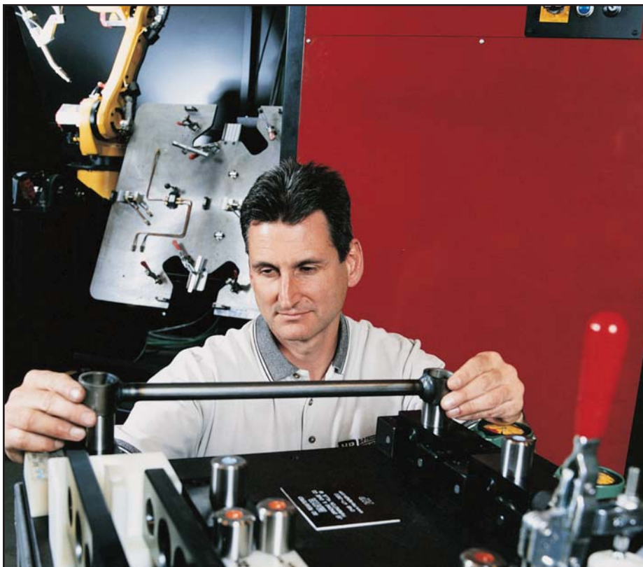
When interfaced with a positioner, complex parts are quickly welded downhand.
