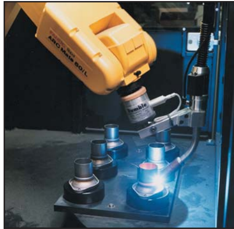
With one setup, six parts are welded
