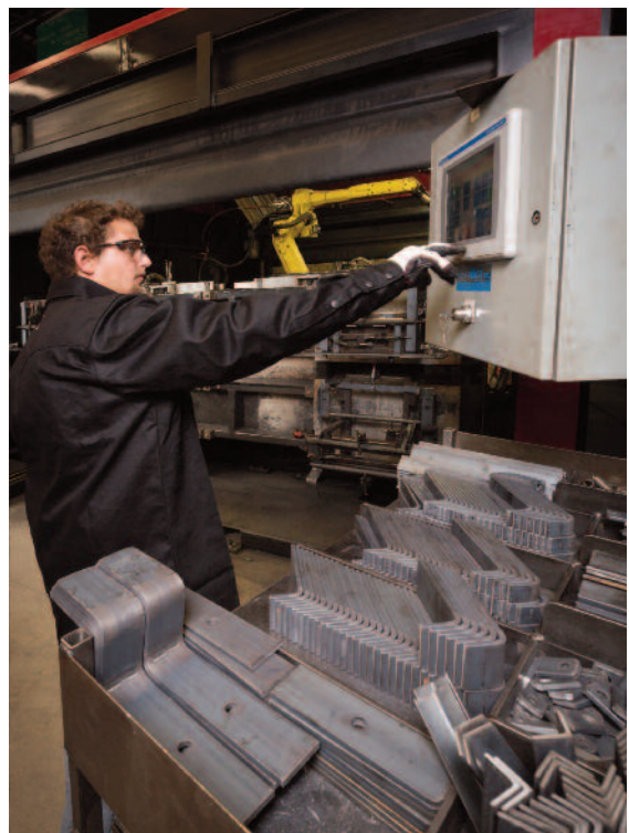
Cotterman personnel evaluates the robotic welding cell system controller.
