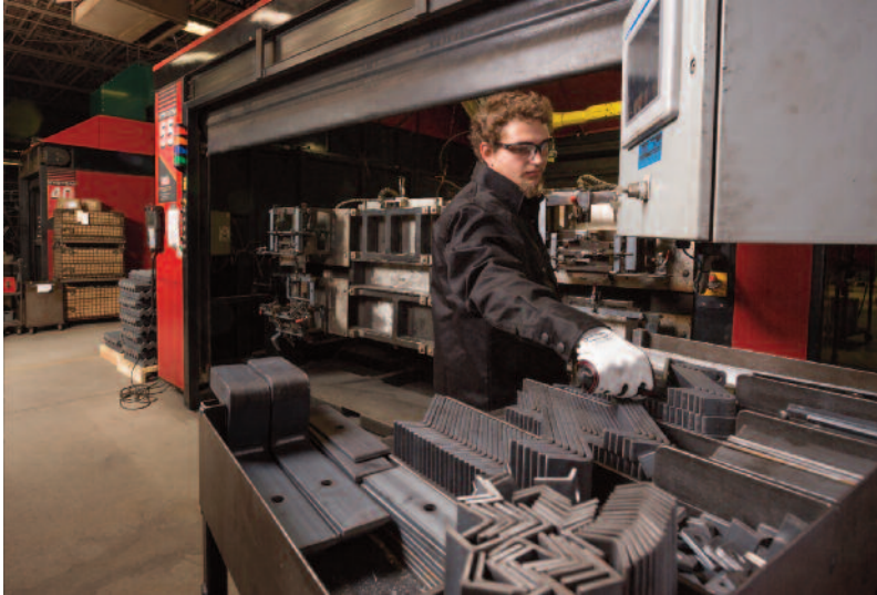
Cotterman personnel loading the System 55 robotic welding cell with smaller common parts.
