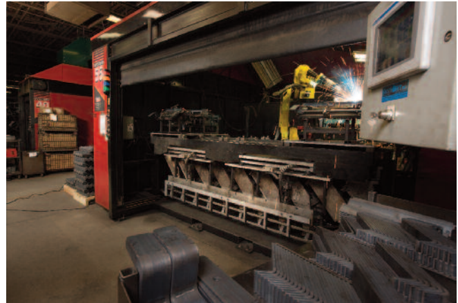
Side B of Lincoln Electric Automation’s System 55 robotic welding cell utilized for welding common parts, multiple fixtures and smaller parts.
