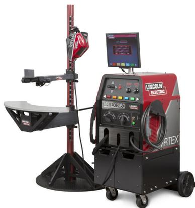
The VRTEX® 360 virtual reality arc welding system allows students to try different welding processes in a variety of simulated welding environments.
