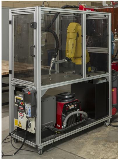
The compact Robotic Education Cell includes a fully functional welding robot that can be used to train students on the set up, operation and troubleshooting of robotic welding and programming.
