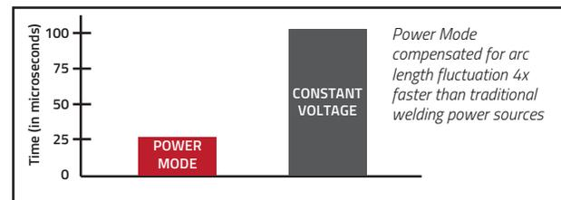
*Power Mode compensated for arc length fluctuation 4x faster than traditional welding power sources*
