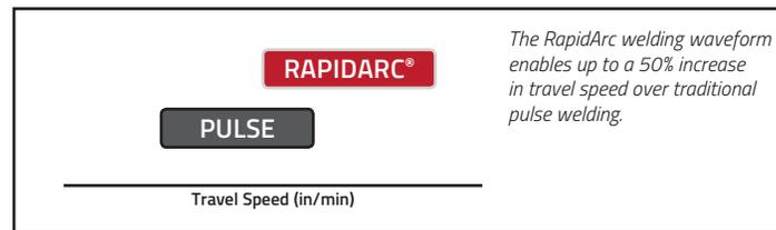
*The RapidArc welding waveform enables up to a 50% increase in travel speed over traditional pulse welding.*
