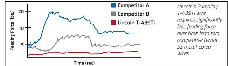
*Lincoln's Primalloy T-439Ti wire requires significantly less feeding force over time than two competitive ferritic SS metal-cored wires.*
