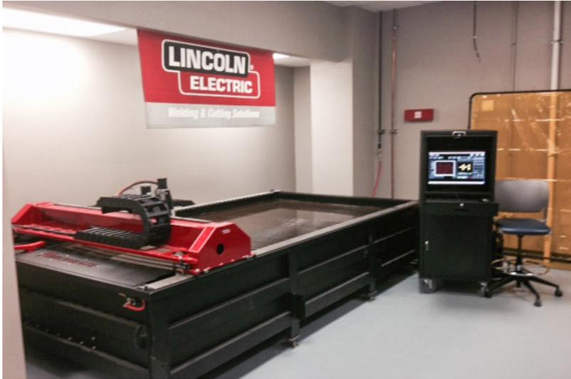
*An industrial CNC plasma cutting system allows students to practice design and programming skills to cut complex 2-D shapes on sheet metal or plate.*
