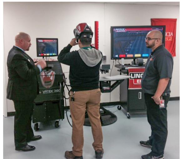
*Virtual reality welding simulators score weld performance and help identify trouble spots in each student's welding technique.*
