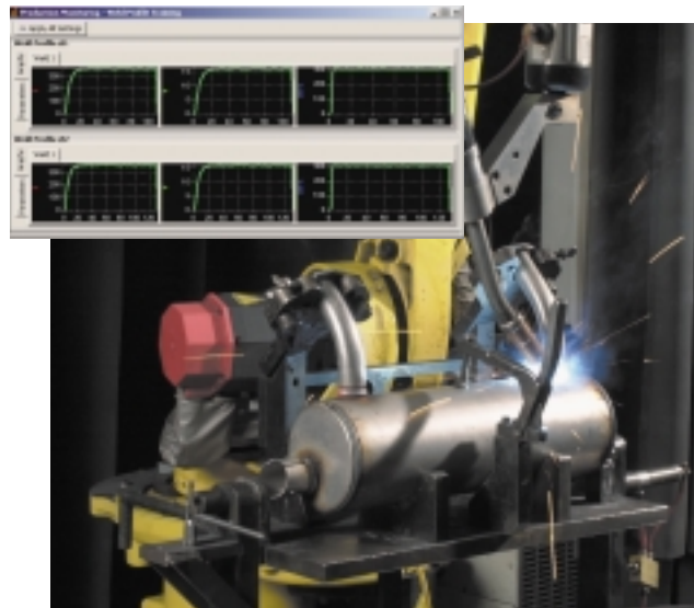
Run a test weld of the second weld profile
