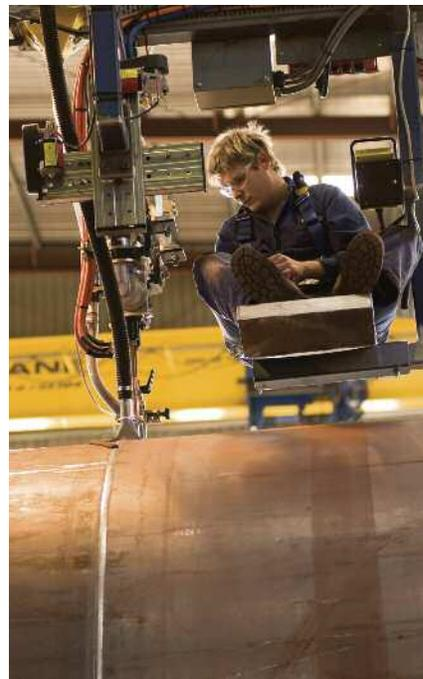
Keppel Prince more than doubled their sub arc welding capacity and increased overall productivity with the Power Wave® equipment platform.
