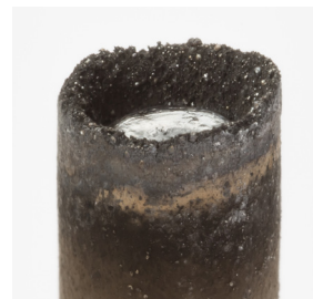
Ideal square burn-off with Pipeliner Arc 80
