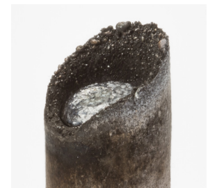
Uneven burn-off with competitive electrodes requires more arc manipulation and results in a poor weld
