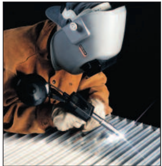
The Magnum® SG Spool Gun is an excellent choice for aluminum sheet metal welding.
