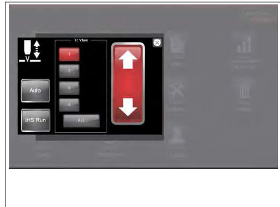
Torch Height Control (THC) Panel
