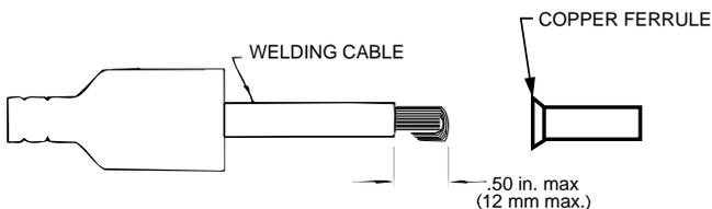
6. Slide the copper ferrule into the brass plug.
