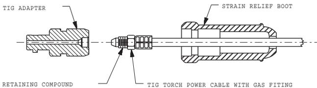
Turn the Power Switch “OFF”. Connect the torch cable quick connect plug into the DC- Output Receptacle on the front of the welder and turn it clockwise until it is tight. This is a quick connect terminal and also provides the gas connection for the shielding gas to the torch.
