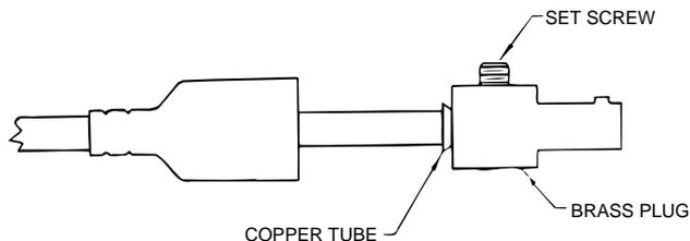
8. Slide rubber boot over brass plug. The rubber boot must be positioned to completely cover all electrical surfaces after the plug is locked into the receptacle.
