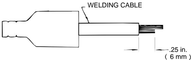
5. Fold copper strands over cut strands and insert into ferrule.
