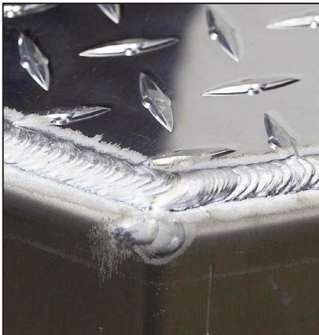
a majority of the parts are being tacked and fed to the robot. The doors are 100 percent welded by the robot, including on the door corners using STT® and for the door stiffeners and stainless steel hinges using the RapidArc® process.
