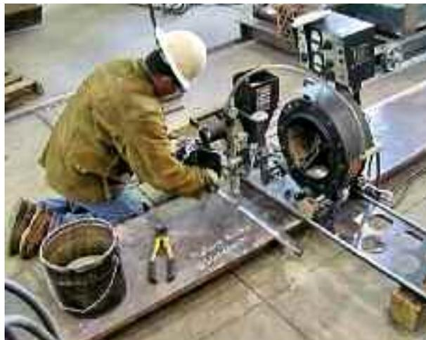
Stinger Welding fabricator uses Lincoln's LT-7 wire feeder tractor for maximum mobility when subarc welding 12 bridge girders.
