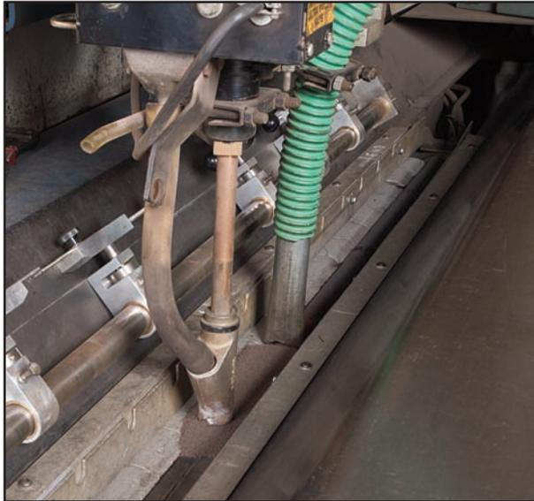
The manufacturing process includes submerged arc welding for the longitudinal and circumferential seams of these vessels. Because of the type of materials they house, the containers also go through a rigorous inspection process, including real-time x-ray to examine the integrity of the longitudinal welds immediately after the welding process and pressure testing upon completion of the tanks.
