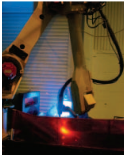
Two six-axis robot arms perform full penetration MIG welds on structural steel—perhaps a first in the U.S.
