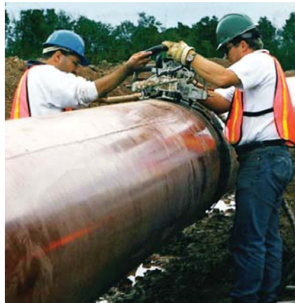
Figure 3: Automated ultrasonic testing (AUT) inspection of pipeline field girth weld.
