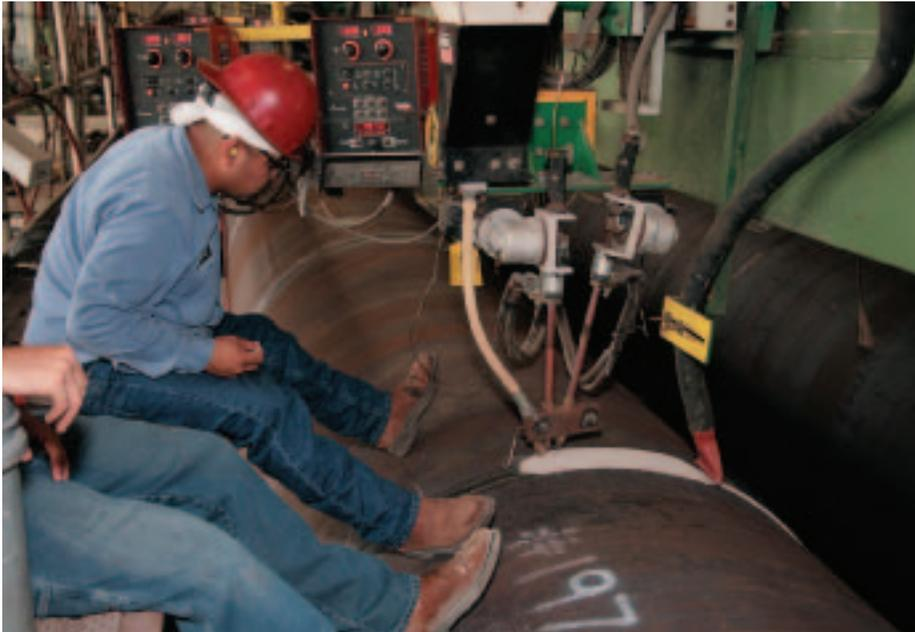
Lending the project an additional hand was Lincoln's Lincolnweld® LA-75 submerged arc wire electrode. Paired with Lincolnweld 880M flux, the wire was specifically selected to maintain or improve travel speeds at these higher amperages while delivering improved mechanical properties.
