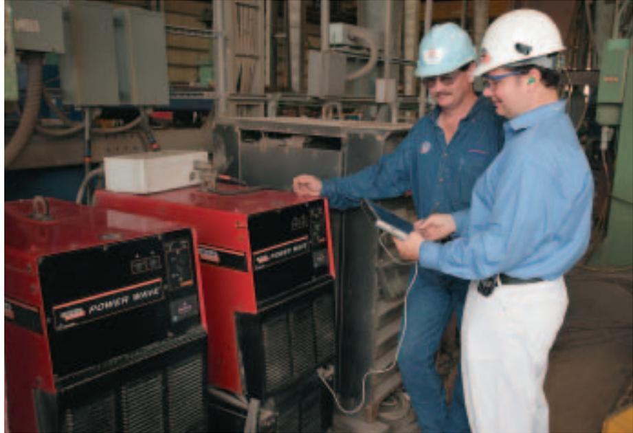
Wave AC/DC, polarities and waveshapes can be changed via software on the fly with a much greater degree of control, allowing the welder to optimize the penetration profile while maintaining the highest possible deposition rate.
