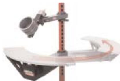
Weld Table can be moved to away position to simulate real life welding applications.
