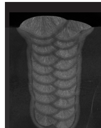
Photo: Offshore narrow groove result. Exceptional performance in demanding offshore joint configurations.
