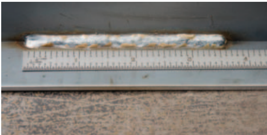
Fig. 4 — The heat input is calculated by taking the final energy value and dividing it by the length of the weld.
