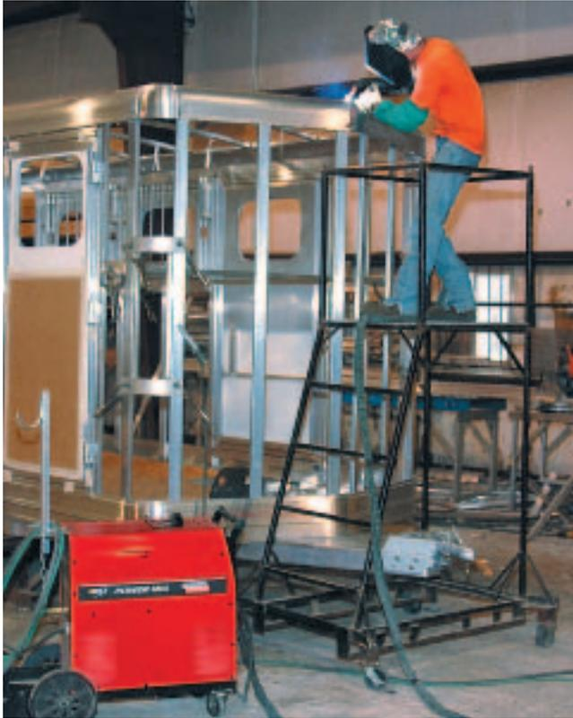
The Power MIG 300 is operated with one-knob synergic control, allowing users to set parameters such as wire feed speed. The unit will automatically adjust itself to the corresponding proper voltage and will constantly monitor the changing characteristic of the arc, making the unit easy to use, even for the novice welder.
